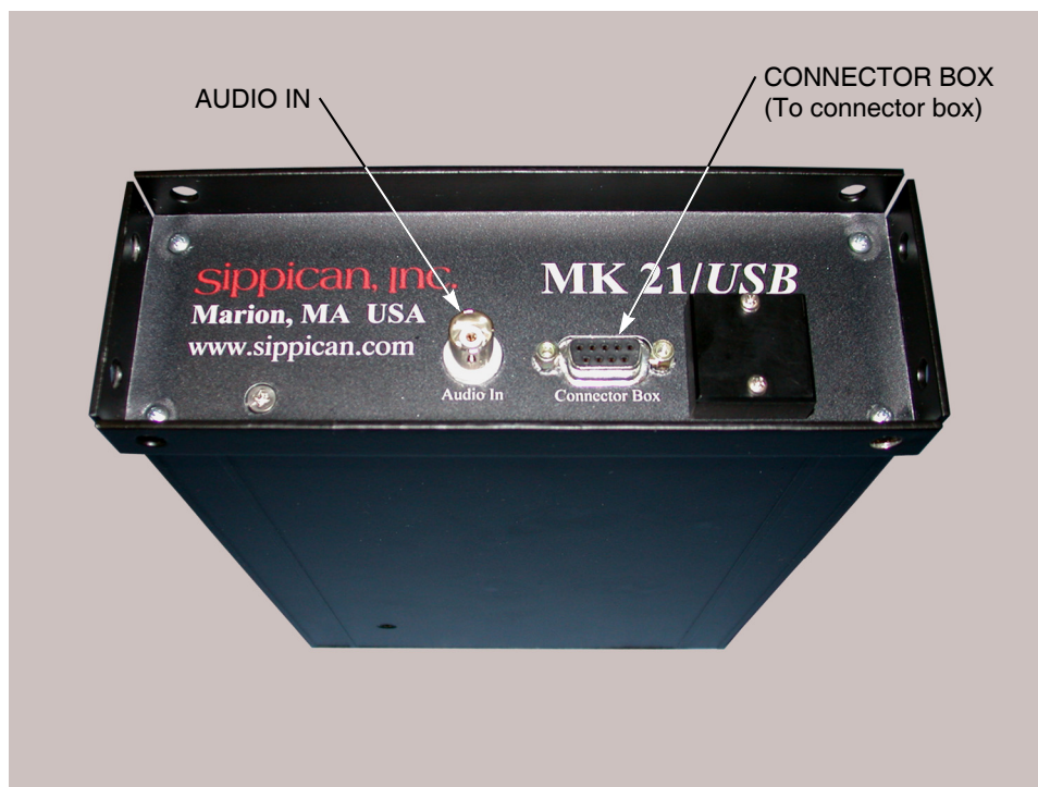
FIGURE 1-6: MK-21/USB Desk Unit Front Panel Audio and Connector Box Connectors
