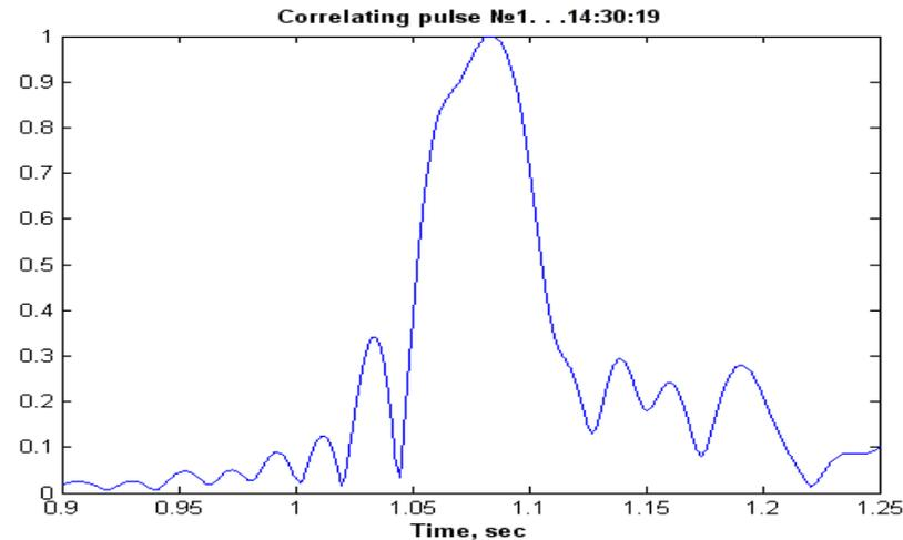
Typical match-filtered received pulse. We see modal decomposition due to intermodal dispersion. Time interval between maximums  $\sim 25$  ms corresponds to interval between the 1<sup>st</sup> and the 2<sup>nd</sup> modes for given distance. In the second figure maximums are not resolved
