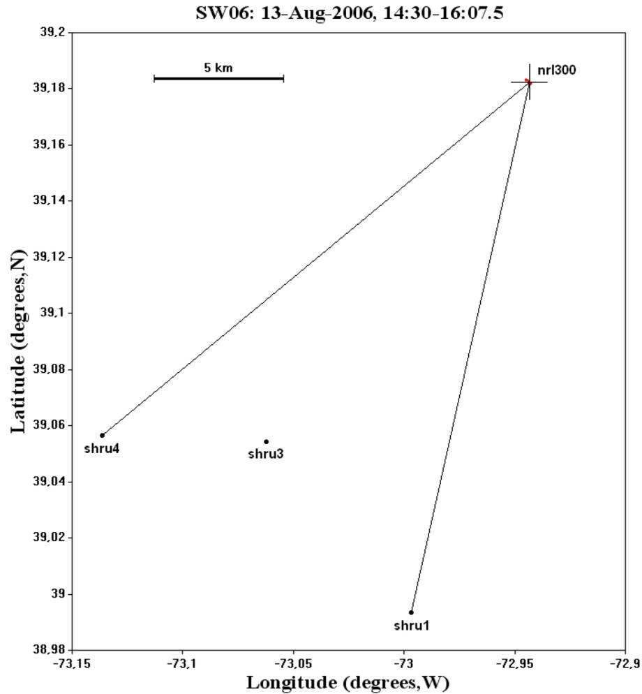
Scheme of positioning using arrival times from two receivers (SHRU1 and SHRU4). Red spots denote are of positions
