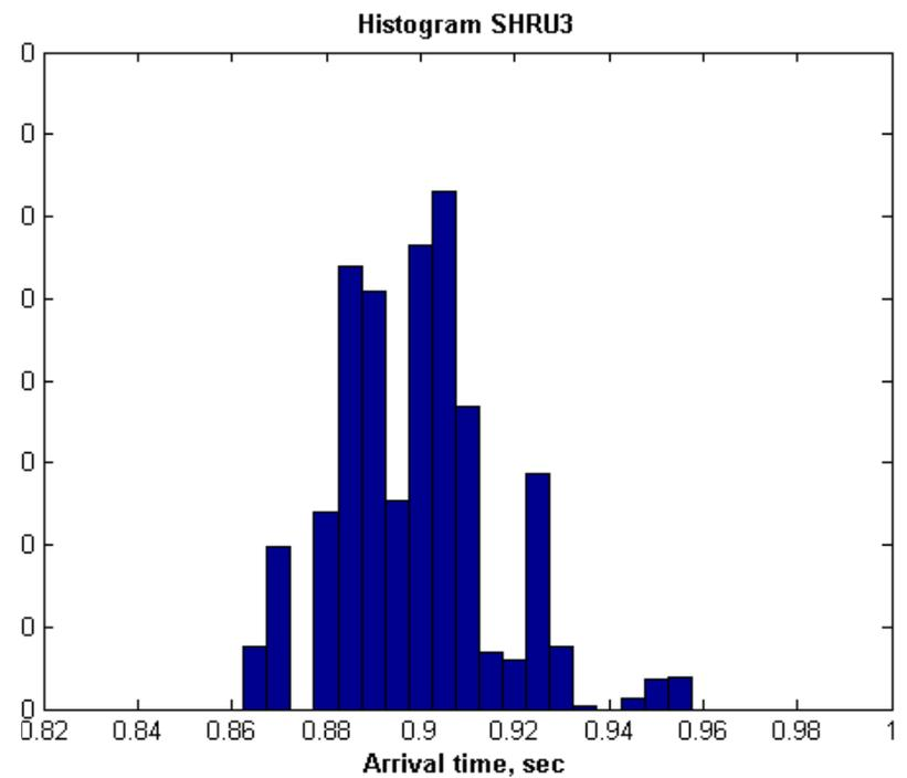
So we have comparatively unstable pulses at SHRU3 in comparison with SHRU1. Remark that in many modes propagation we see significant fluctuations of temporal position of global maximum. Accuracy to position of the separate mode is  $\sim 0.01$  sec. Histograms are made using 1980 pulses during  $\sim 8.5$  hours.
