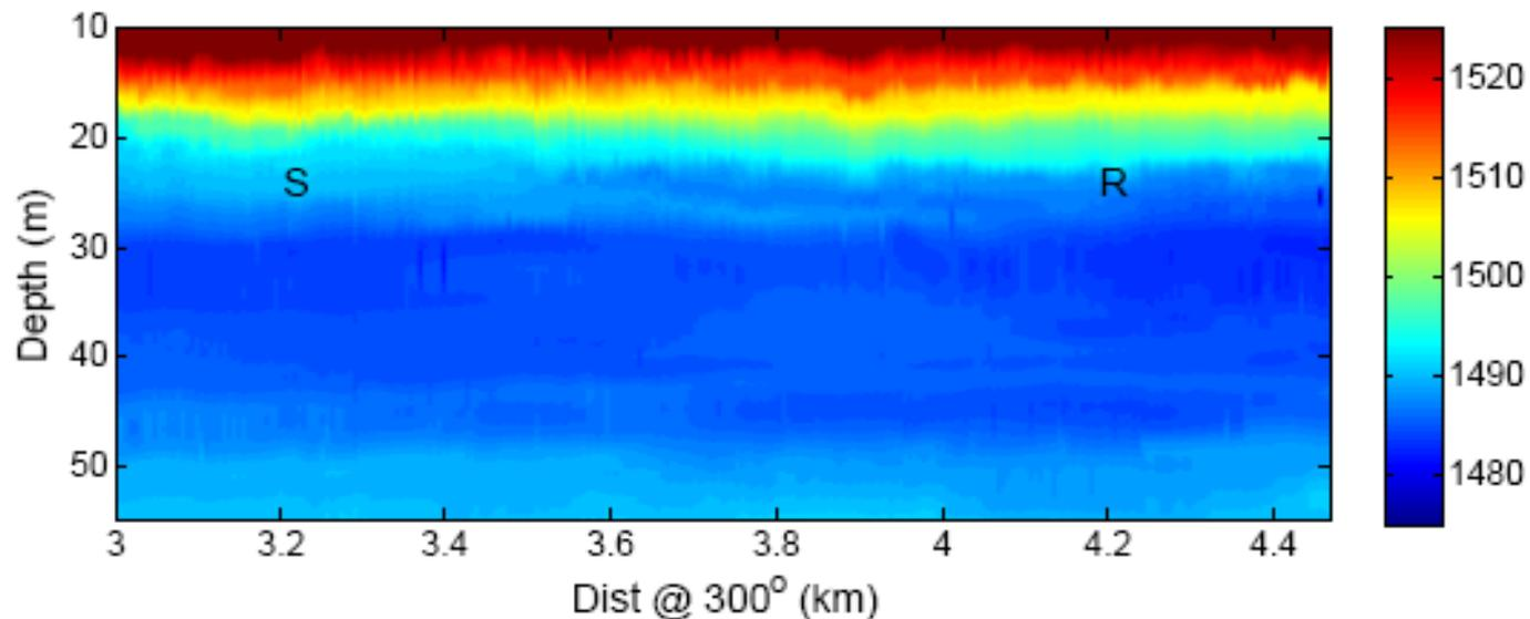
Sound Speed Profile and range-independent ray tracing to 2 km:
