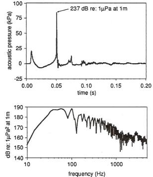
A typical CSS pressure signature (produced by the combusion of 5.0 I stoichiometric hydrogen and oxygen and the power spectrum
