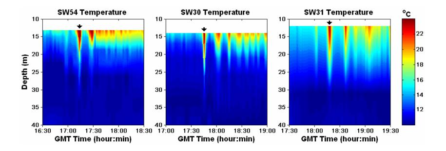
In supposition of constant velocity of internal waves it is possible to construct space distribution of temperature, for example for 15:31 GMT along a straight line between thermistor's sensors SW24 ± SW23 ± SW54. Black arrow denotes position of the soliton at 16:20 GMT
