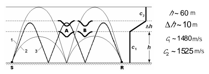
Interaction of ray with the moving perturbation at the position A is greater than at the position B. So temporal fluctuations of intensity from the source S at the receiver R take place.
