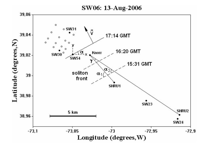
Source is at the R/V Knorr, receivers are SHRU1 and SHRU2, waves fronts of the first peaks in the train are shown for 16:20 and 15;31 GMT  $\gamma \sim 15^{\circ}$
