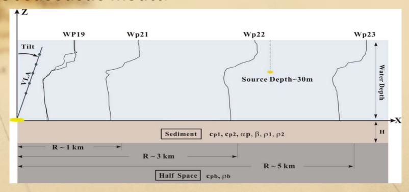
Geometric parameters: 4 (WD, R, SD and VLA tilt)
